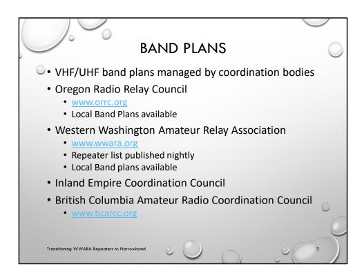
VHF/UHF Band plans are a local option and generally published by the local coordinating bodies. These band plans show differentiate weak signal, satellite, packet, simplex, repeater and crossband repeater areas.
