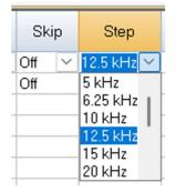
TStep is one of the fields available when programming a channel in CHIRP. Step is visible in other software as well. Internally the radios store the frequency information as a binary value with a
