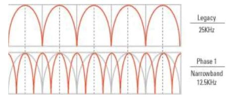
The existing 2m band has 20kHz channels which does not divide into 12.5kHz channels evenly. The diagram below is an approximation of how the existing and new narrow channels will appear. This is just a small portion of the spectrum but it is possible to see that some (~20%) of the new channels line up with the old channels. The remaining systems need to move at least a little.
