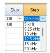
TStep is one of the fields available when programming a channel in CHIRP. Step is visible in other software as well. Internally the radios store the frequency information as a binary value with a
